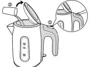
3. Close the lid, put the kettle on the power base and insert the power plug.
